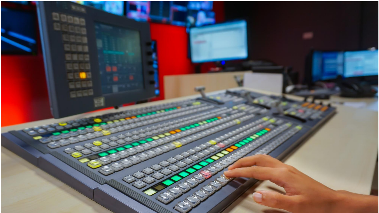
—Professional hardware vision mixer in a TV control room
