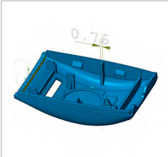
Figure 8: Optimization of the wall-thickness during the mechanical engineering phase to increase manufacturability.
