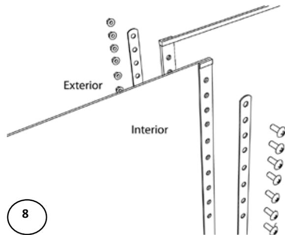
When tightening the screws start from either the top and go down or vice versa. Do not start a few screws from top and a few from the bottom to meet in the middle, this can cause problems later on.
