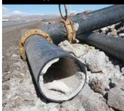
Figure 3. Dissolved solids precipitated scale in a brine transfer pipe
