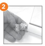
Fit plunger lock on end of second shoe section and secure with set
