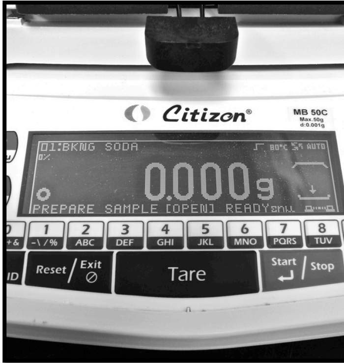
Make sure to tare the empty pan weight before loading sample
