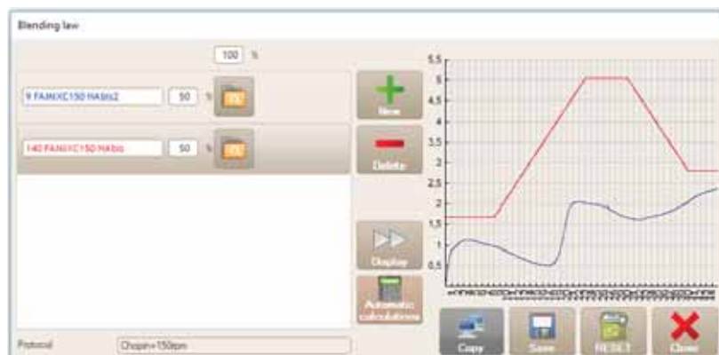
Figure 18: Blending tool – Virtual curve of the resulting flour blend
