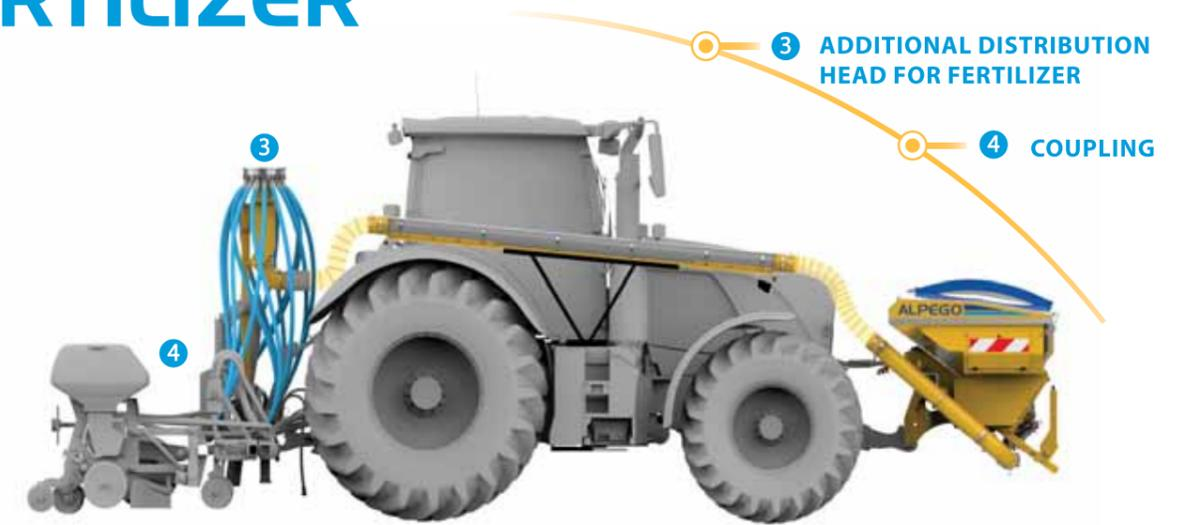
The fertilizer configuration, with a dedicated distribution head, provides the front hopper in combination with various machines: weeders, precision seed-drills, cultivators, rollers, etc ...
