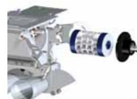
**1 REPLACEMENT OF THE METERING UNIT ROLLER**
