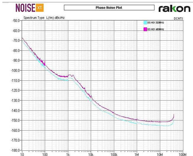
Fig 15: Phase Noise @ 320 and 480 MHz with internal DDS clock
