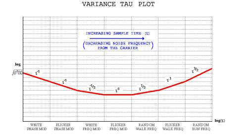
Note:- This plot is a log / log plot (Noise source legends are shown reversed compared to the Spectral Density Plot ).
