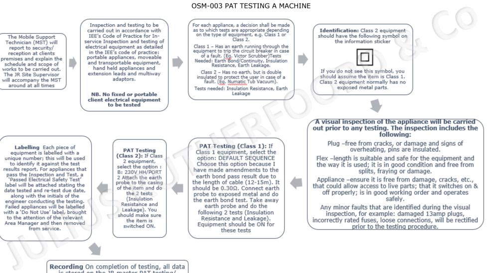
Recording On completion of testing, all data is stored on the JR master PAT testing/ inventory records and site specific data can be generated where needed
