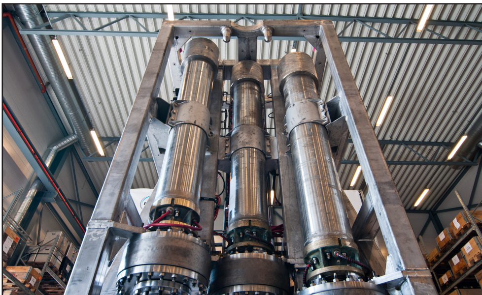
Detail of EC-Drill® pump in the Enhanced Drilling workshop, Straume, Norway
