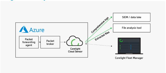
The Corelight Cloud Sensor deploys as an Azure VM Image instance and ingests mirrored-traffic from a packet-forwarding agent. After making a few simple config changes in Corelight's management console the sensor will export data to downstream storage and analytics tools such as SIEMs or file analysis platforms. Corelight offers export controls, such as log fork and filter and fleet management capabilities for multi-sensor environments such as policy templates
