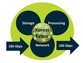
• **Xpress Fabric** – A switched PCIe fabric with 160 dynamically configurable PCIe lanes, allowing for 240 Gigabytes per second or 1920 Gigabits per second of total throughput for efficient communication between processor and peripherals.
