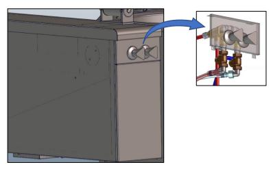
**Repreparation:** Disconnect hot-and cold water from the unit. Remove top cover and front cover. Also side cover if necessary.
