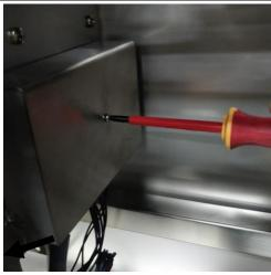
3. Connect wire nr.1 to Connection X4:1.Use Pancon tool for connection wire to the connector
