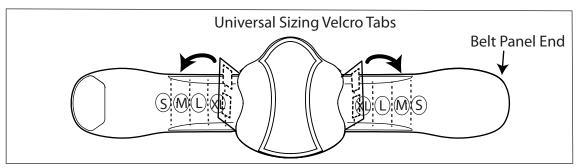
1. Adjust universal sizing by moving panels through D-ring to the desired size. Size markings are clearly labeled on the inside of each panel. Align and firmly secure each panel by attaching the hook to loop area.
