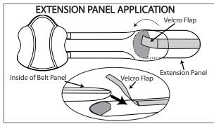
If patient requires a larger size than universal, an Extension Panel is available to add 18 inches in length (70 inches in total girth). The Extension Panel attaches to the outside of the left belt panel. The velcro flap of Extension Panel should attach to the inside of the belt panel.
