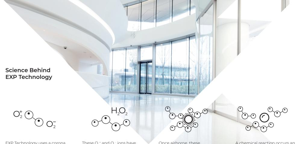
EXP Technology uses a corona discharge system to generate Oxygen ions  $O_2^+$  and  $O_2^-$  at a high density.
