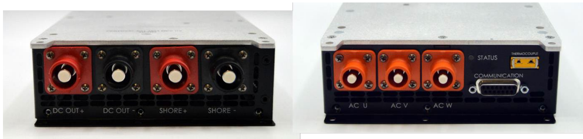
Figure 2: The iPS (PMU) takes AC inputs from the SG (right) and converts to DC outputs (left). The communications port is the CAN interface.
